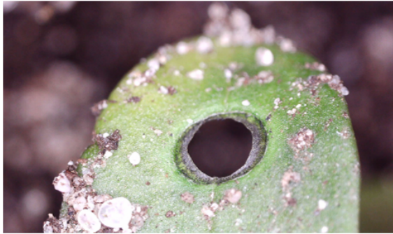
100W Blue Diode Laser firing with 30ms pulse, © Laser Electronics LE GmbH
